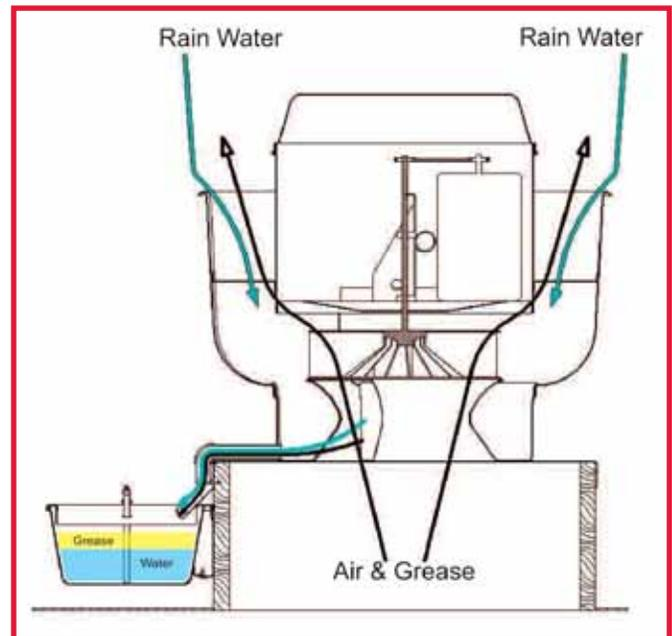
The Interceptor separates the grease from the water. The liquid grease remains in the Interceptor and clean water flows freely out of the unit.
